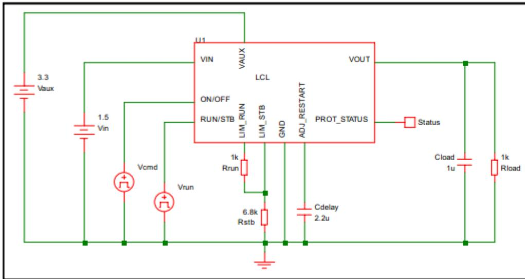
Case 2: Vin voltage is equal to 3.3V. Internal circuits are also powered from Vin. Ith\_stb is set to 0.2A. Ith\_run is set to 1.2A. Delay is set to 85ms. ON/OFF state and RUN/STB mode are selected by dedicated commands.
